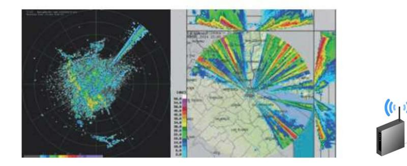
Figure 7.19. The image on the left demonstrates the type of expected interference from a Radio Local Area Network located 6.4 km away at 0.42° elevation angle. The image on the right is from an operational weather radar, courtesy of Claudia Campetella of the Servicio Meteorológico Nacional (Argentina).
